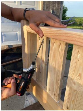
Step 1: Build the frame of the swing. Using a Mitre Saw, cut the 4x4 and the 2x6 boards to length. Build the base frame of the swing, the 2x6 should be centered on the 4x4. Use two of the structural wood screws for each board. A speed square helps to line up your boards.
