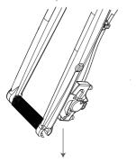
B. Remove the plastic insert card from the front brake caliper.
