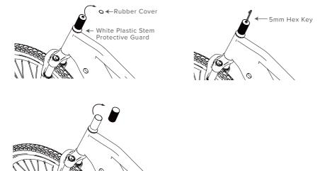
B. Place the handlebar stem onto the stem with the display facing upwards, replace the top cap and use a 5mm hex key to secure the handlebar stem. Reinsert the rubber cover back into the top cap.
