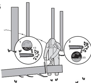
When the log is supported on both ends, as illustrated in Figure 6, cut 1/3 the diameter from the top (overbuck)(1). Then make the finished cut by underbucking(2) the lower 2/3 to meet the first cut
