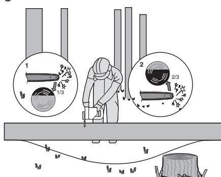
When bucking on a slope always stand on the uphill side of the log, as illustrated in Figure 7. When "cutting through", to maintain complete control release the cutting pressure near the end of the cut without relaxing your grip on the chain saw handles. Don't let the chain contact the ground. After completing the cut, wait for the saw chain to stop before you move the chain saw. Always stop the motor before moving from tree to tree.
