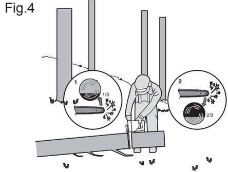
When the log is supported on both ends, as illustrated in Figure 5, cut 1/3 the diameter from the top (overbuck) (1). Then make the finished cut by underbucking (2) the lower 2/3 to meet the first cut.
