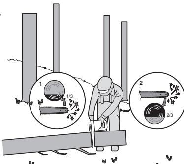
When the log is supported on both ends, as illustrated in Figure 5, cut  $\frac{1}{3}$  the diameter from the top (overbuck) (1). Then make the finished cut by
