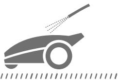
Landroid Vision is IPX 5 waterproofed and can be washed by using a regular garden hose.
