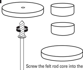
Screw the felt rod core into the felt
