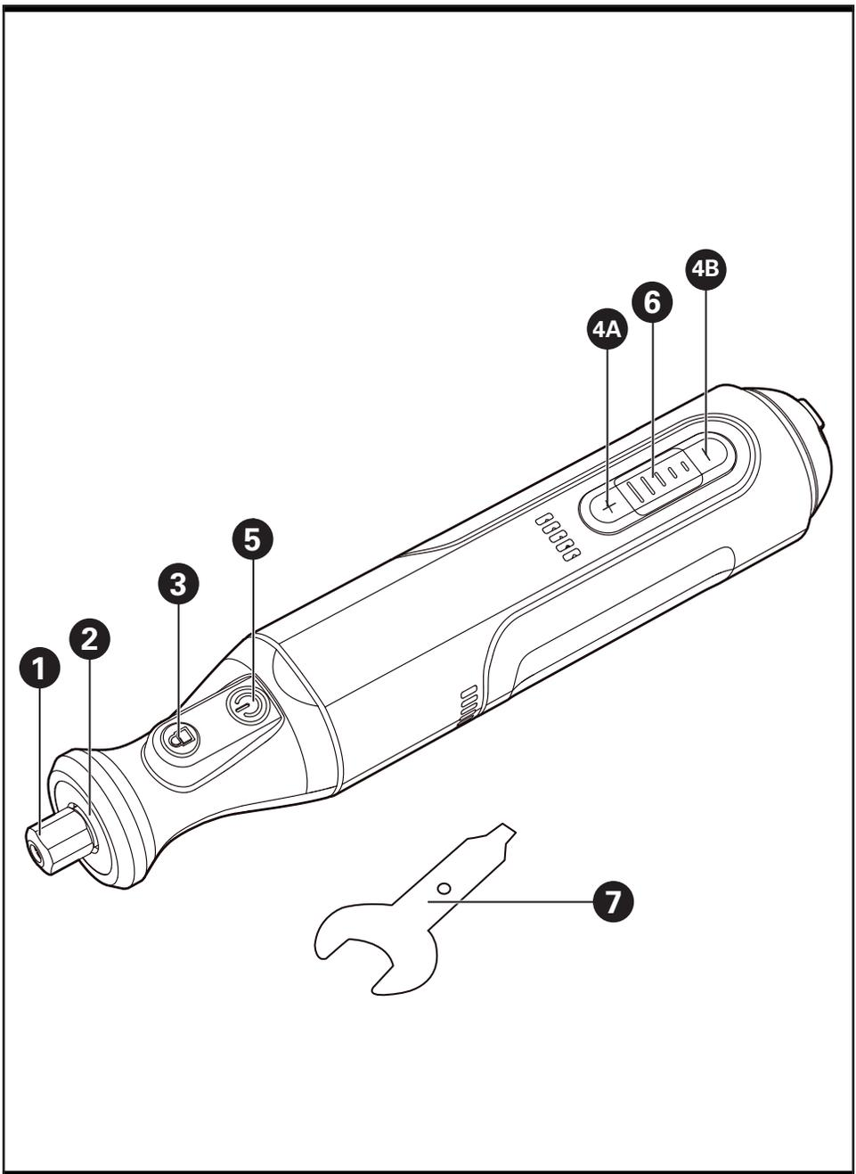
**1. COLLET COVER****2. LED WORK LIGHT****3. SPINDLE LOCK****4A. SPEED ADJUSTMENT BUTTON "+"****4B. SPEED ADJUSTMENT BUTTON "-"****5. ON / OFF BUTTON****6. SPEED INDICATOR / BATTERY INDICATOR****7. CHUCK WRENCH**
