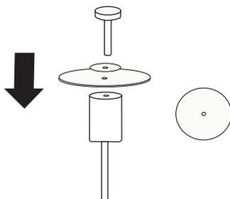
Installation of the cutting blade
